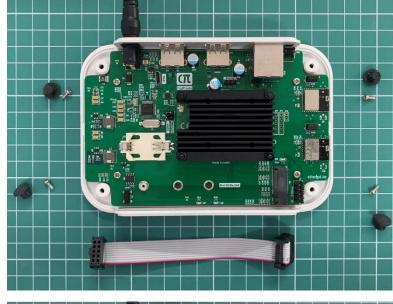
Place the connector and fit on P6 as shown in next image.
